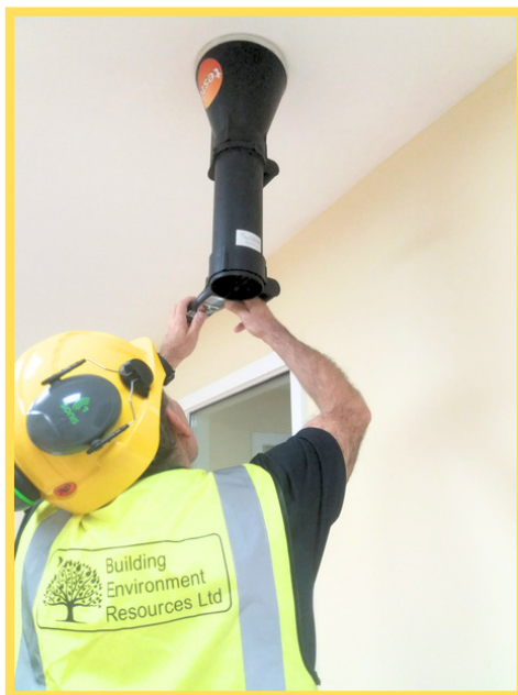
Our ventilation engineer testing flow rates to I.S. EN 14134: 2019:
