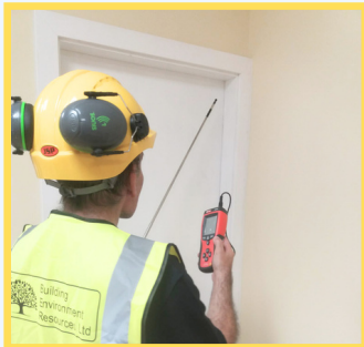
Air testing engineer quantifying the air leakage through an external door
